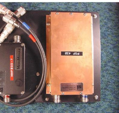
The 70cm/2m **duplexer** is a handy “compromise,” which can be used alone if either of the filters in figure 1 are unavailable.
